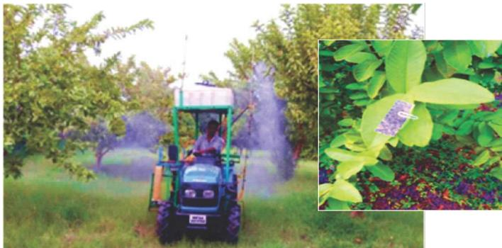
time of the spraying system were 475 l/ha and 12 s, respectively. The volume mean diameter (VMD) and volumetric spray deposition were 248 µm and 0.291 µl/cm<sup>2</sup>, respectively.
