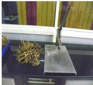
parts of roots. . The de-bunching capacity of the developed tool for *Safed musli* was 10.3 kg/h as compared to 5.1 kg/h for manual de-bunching without knife and 7.5 kg/h with knife. The percentage of separated roots and material loss were recorded as 84 and 16 %, respectively for de-bunching of *Safed musli* roots using the tool. The tool increases de-bunching capacity by 2.8 kg/h and reduces material loss by 4 % over traditional practice.
