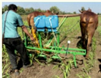
opener is 0.19 and 0.30 ha/h, respectively. The average discharge from each nozzle is in the range of 195.9 and 197.6 ml/min. The uniformity coefficient of the sprayer has been observed as 74% with weeding efficiency of 84% in soybean.
