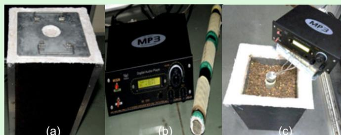
Acoustic insect detection system (a) Acoustic shielded bin, (b) Signal processing system and Sensor Probe, (c) Probe installation view
