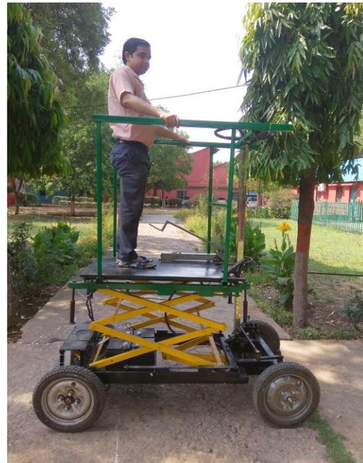
power pack and has provision of moving forward, backward and height adjustment using a hydraulic system. The force and energy required to move the platform is 59 N and 600 Nm, respectively at a forward speed of 0.54 km/h. The energy required to lift platform for change of stage (0.4 m) is 400 Nm. It has gear ratio of 1:9, lifting per stroke of 0.15 m with a total lift of 1.2 m.
