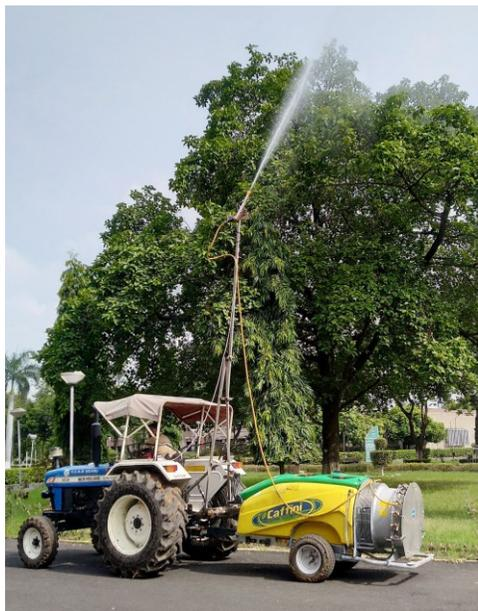
spray deposits per square meter and volumetric spray deposition are 11%, 302 deposits/m<sup>2</sup> and 0.55 µl/cm<sup>2</sup>, respectively. The approximate cost of the retrofitted spraying system is ₹ 18,000/-.
