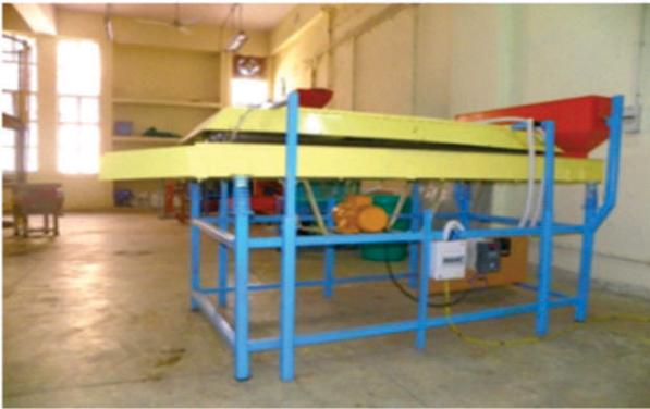
required for loosening of biological bonds prior to milling. Hydro-thermal treatment is the most common and commercially used for pigeon pea. But, it is time and energy consuming, expensive and have some other quality and safety issues. Therefore, a controlled infrared radiation based pre-treatment system has been developed to reduce time of milling and cost.
