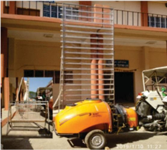
sensitive paper (WSP) is attached to the grid of 250×250 mm for measurement of droplet size on the platform and tested at different forward speed during commercial testing of sprayers. The wind velocity can be measured at the centre of each grid by placing a hand held anemometre at the centre of each grid and data is recorded.
