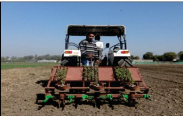
(disc type), seedling tray shifter, seedling trays, ground wheels and chain and sprocket type power transmission system. The average field capacity, field efficiency, labour requirement and fuel consumption of transplanter are 0.11 ha/h, 56%, 18 man-h/ha, and 3.5 l/ha, respectively; whereas, transplanting efficiency and overall efficiency are 92% and 85%, respectively, for tomato and chilli seedlings at the forward speed of 1.2 km/h.
