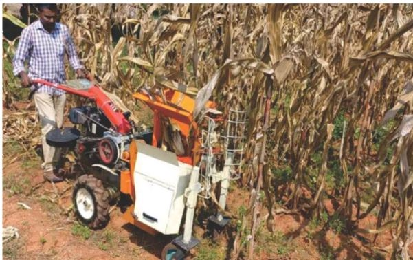
capacity is provided at the side of the machine to collect the cobs. Two wheels are provided at the front to facilitate the movement of the harvester in the furrows. The effective field capacity of the harvester is 0.2 ha/h and the cost of operation of the maize harvester is Rs. 2850/ha. The saving in cost of operation, time and labour are 25, 96 and 91%, respectively as compared to manual harvesting.
