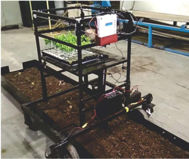
The developed robotic transplanter is operated by 12 V battery and can pick up and transplant about 3 seedlings/min. The success rate, leakage rate and successful transplanting were about 95%, 7.6% and 90%, respectively for 30 days old chilli seedlings. The potential use is to enhance input use efficiency for sustainable productivity and reduce drudgery by avoiding manual practice.
