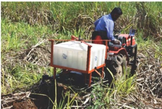
The equipment has been tested at farms of ICAR-Sugarcane Breeding Institute, Coimbatore and M/s. Bannari Amman Sugars Ltd., Sathyamangalam, Erode district in Tamil Nadu. It applied EPN solution at the rate of 30-32 Infective juveniles/ml (IJs/ml) from each outlets at root zone of sugarcane crop to control white grub and has an effective field capacity of 0.18 ha/h. The cost of operation of the equipment is ₹ 2550/ha and results in cost saving of 47% as compared to manual method.
