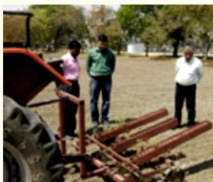
and save the time. The metering mechanism has been preliminarily evaluated in the field. The speed of operation of the machine was found to be 1.5 km/h.
