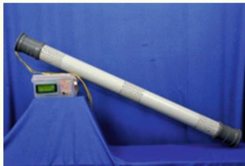
Sensor rod mounted with alert generation system
