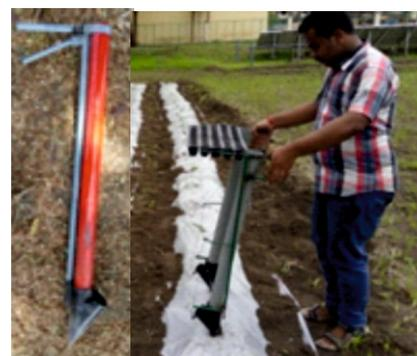
**Model 2- Two row:** The two row unit consists of portray fixing arrangement, two delivery pipes, frame with clutch and handle and jaw type mechanism. The transplanter has an overall dimension of 530 x 610 x 1000 mm, weighs 5 kgs and costs Rs 1000
