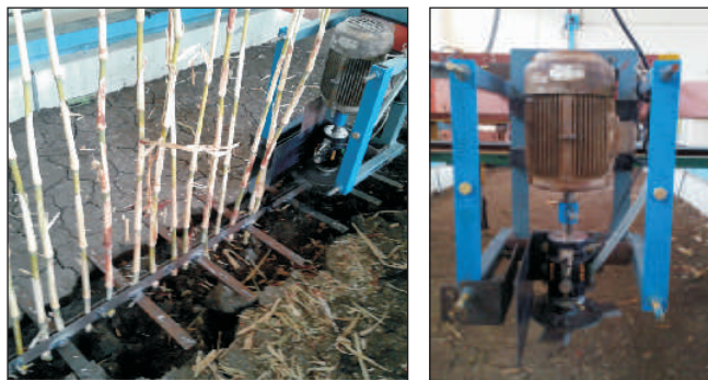
Fig. 8: Setup for torque measurement
