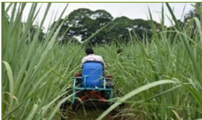
diluted EPN solution is pumped by using battery operated diaphragm pump with the output capacity of 4 l/min. The solution outlet is taken from the bottom side of the tank through pump to behind of the furrow opener. The capacity of the tank is 75 l. The field capacity of the equipment is 0.16 ha/h at an operating speed of 2 km/h. The savings in cost of operation is 70%. Saving in labour is 85 per cent.
