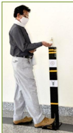
of sanitizer or liquid soap can be dispensed by pressing the foot pedal. Total height of the unit is 1100 mm. It is portable and can be placed at entrance of lobbies, corridors, farms, meeting rooms, outside the shops etc. The cost of this unit is about ₹ 1000/-. This developed unit is being used for hand sanitization at different premises of the institute.
