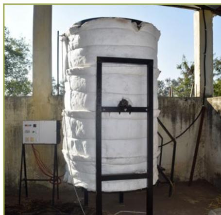
Torrefaction experiments were carried out on paddy straw to investigate the biopolymeric changes in crop residue when the biomaterial is heated until temperatures of 200–300°C and
