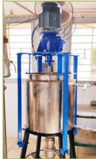
process. The pilot plant unit is capable of extracting dietary fibre from both soybean hull as well as chickpea hull with a capacity of 10 kg per batch and extraction efficiency of 80%. The biochemical analysis shows the total dietary fibre content of extracted dietary fibre from soybean hull and chickpea hull as 80% and 76%, respectively. The total cost for the establishment of dietary fibre extraction pilot plant is worked out as ₹ 2,96,400/- and
