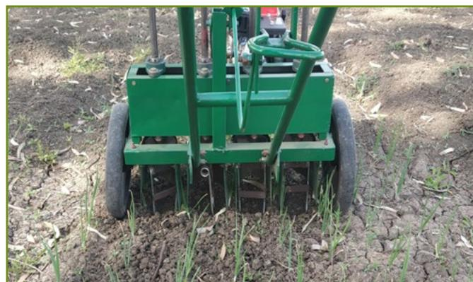
damage with the push type weeder are 91.21% and 6.81%, respectively. Push type onion weeder has been upgraded to self-propelled weeder by giving power from same 1.12 kw petrol engine to the wheels. Performance of weeder is found satisfactory during ongoing field trials. However, line transplanting of onion seedlings may be recommended for the best performance of weeder.
