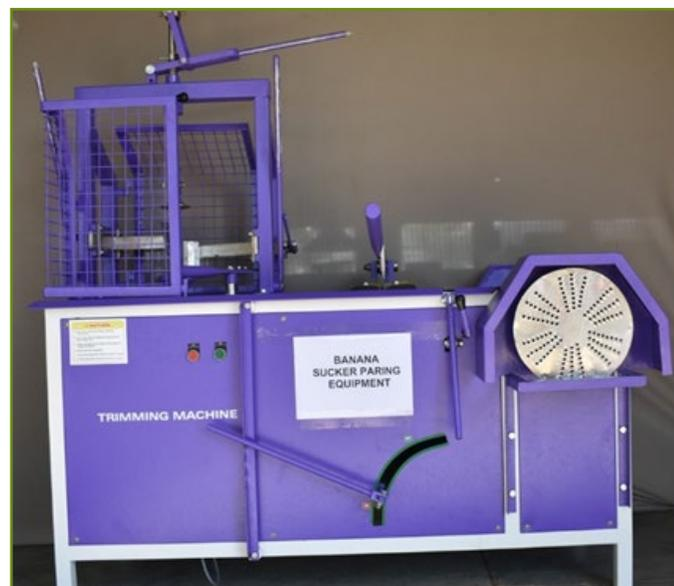
blade and adjusted as per the area and the depth of the banana sucker to be trimmed. The capacity of rotating grating double blade mechanism is about 200 suckers per h. The saving in cost of operation is about 75 per cent.
