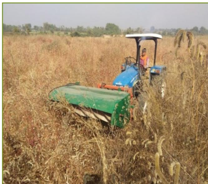
needed for efficient grass seed harvesting. It consists of the spiral bruising element on a rotary cylinder head which act as a grass seed collection mechanism. The machine has been tested in Dinanath Grass field at ICAR-IGFRI, Jhansi and its seed collection capacity found to be 5.5-6.0 kg/h, and the time required to fill the seed collection chamber is 40-45 min. The effective field capacity of the grass seed harvester is 0.1 ha/h at an average operating speed of 3.24 km/h for Dinanath grass.
