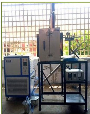
with the monometallic or bimetallic catalyst bed inside the reactor forming gas and liquid products. Both the catalysts were observed to have two stages of weight loss signifying moisture removal and metal oxide formation through thermo gravimetric analysis. Activation energy increased with increase in cobalt addition (9.98 to 10.86 kJ/mol) in bimetallic catalysts implying difficulty in formation of cobalt oxide in the presence of iron.
