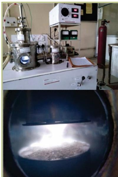
pirani gauge for vacuum pressure measurement, integrated three ways to control the vacuum inside the reactor. It can generate the vacuum as high as 10<sup>-8</sup> bars. The thermal degradation behaviors of crop residues can be studied under different levels of vacuum and plasma intensity in different environment. Generation of free and charged radicals in plasma under different
