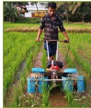
the developed system can be used for 5 different operations viz. wet land paddy weeding, row crop vegetable weeding, shallow tillage, digging small diameter pits and basin clearing for coconut tree. Paddy weeding attachment has also been developed for the multipurpose tool carrier which is powered by the 1.5 kW brush cutter engine.
