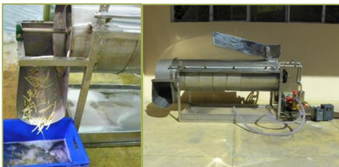
off material. The capacity of machine for *safed musli* peeling is 15-20 kg/h. The machine has potential to mechanize peeling operation of medicinal root crops and to reduce drudgery, labour cost and time.
