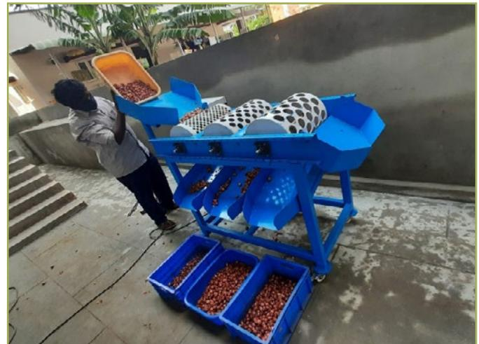
size of multiplier onion. The multiplier onion fed into the feed inlet passes to the rotating grading drums and the graded onion get collected at the respective outlets provided below the grading drums. The capacity of grader is 580 kg/h and is operated by 0.75 kW single phase electric motor.
