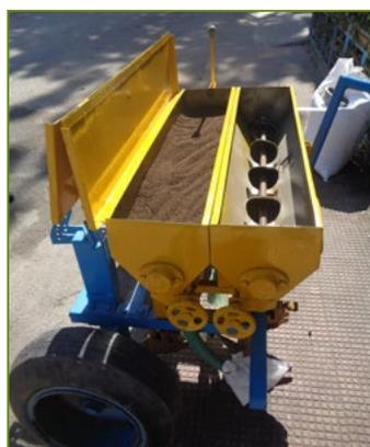
Animal drawn seed cum manure drill developed by MPUAT, Udaipur center consists of a rectangular shaped main frame, screw jacks to vary the height of frame from the ground, two pneumatic wheels and a hitch beam. Furrow openers are clamped on the frame using quick fixing type ‘U’
