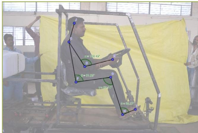
mm) and the range of trunk, elbow, hip, knee and ankle angle and overall dimension of workstation has been made to suit most of the drivers. All the prime mover controls viz. steering, brake, accelerator, etc. are suitably placed within operator reach envelope.
