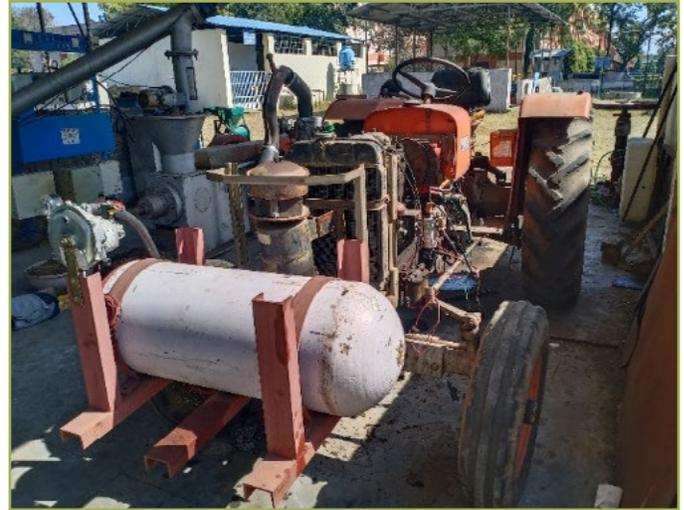
distributor and fitted/aligned in the timing gear mechanism of the tractor with modified flange. An inlet air manifold has been fabricated and carburettor has been suitably fitted to regulate the air-CNG mixture. All the arrangements with air cleaner have been made to connect carburettor and air cleaner. Further arrangements are in progress to operate the tractor engine with 100% CNG.
