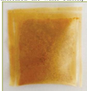
properties. The water barrier property of the film ranged from 5.3 to 9.2 x 10<sup>-10</sup> g/ms Pa. The tensile strength of the film varied from 5.1 to 8.2 MPa, which is higher than similar composite edible films. The elongation of the film ranged from 70 to 88%. The edible film was
