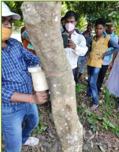
knife or girdling knife which takes around 15 minutes to girdle a branch and girdling depth is also not uniform. Sometimes two to three branches of a litchi tree need to be girdled, which require more time per tree. In order to mechanize this laborious process, a motorized girdling tool has been developed by the institute. It mainly
