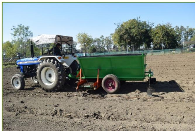
developed equipment is 0.44 ha/h with field efficiency of 80%. The functional testing of the machine has been completed; however rigorous testing in grape orchards will be carried out in next season.
