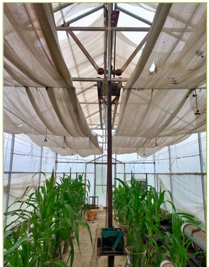
winch machine with rope, pulley, movable unit, and fixed stand. The fixed stand is mounted on the stable platform inside greenhouse. The movable unit is moves up and down on the fixed stand by using the winch machine and pulley. Other parts of the movable unit are attached to the top of greenhouse. The developed mechanism is a manually operated low cost and low maintenance system which is suitable for lifting the top of the greenhouse upto 200 m<sup>2</sup> area.
