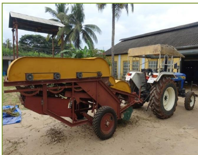
threshing system. The threshing and conveying efficiency of the picker combine is found to be 99% whereas the maximum stripping efficiency is 95% at 4 days after harvesting. It has been observed that, the entire plant mass is picked up by the header and conveyed into the threshing cylinder without any damage to kernal and pods.
