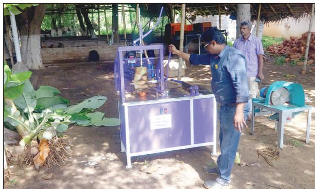
roots before placing it on the holder for trimming. The equipment is best suited for large size suckers. The capacity of the equipment is about 120-150 suckers per hour, the overall size of the equipment is 1145 × 515 × 1825 mm. The cost of the equipment is Rs. 80,000/-.
