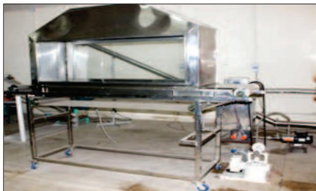
drying section, for visual inspection. An exhaust fan provided at the top of the drying cabinet ensures expulsion of water vapour removed from the drying material so as to prevent condensation of vapour. Wheels are provided at the base of dryer frame for its easy movement.
