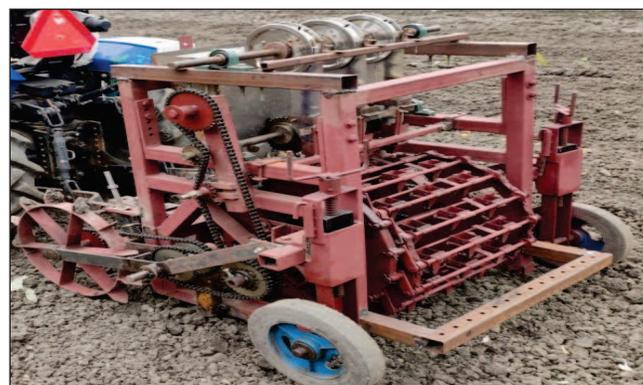
arrangement. Leveling roller is attached to the main frame in the front of the dibbling unit for leveling the soil and providing the uniform soil surface to the cups of dibbling unit. The chain and cup-type metering unit is being fabricated for picking the garlic cloves from the seed box and dropping in to the cups of dibbling unit. Precision planting with minimum losses of seeds can be done with this machine to achieve the higher productivity of garlic.
