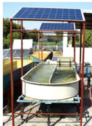
60 V and 6.9 A, respectively. Time required for harvesting is 4 h to bring down optical density of microalgae from 0.98 to 0.16 and harvesting efficiency varies from 81 to 86% during the different harvestings throughout the year. Average energy consumption for electro-flocculation is found to be 3 kWh/kg of dry microalgae biomass.
