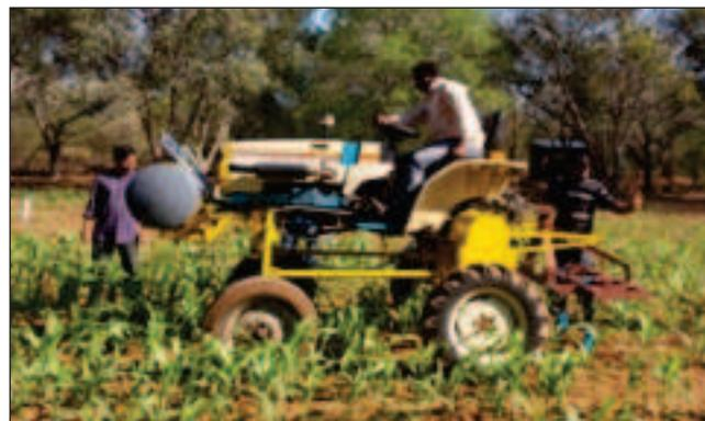
tasted in castor, pigeon pea and maize crops. The weeding efficiency of rotary weeder is found to be 82.5%. The approximate cost of the machine is Rs. 30,000/- and its operating cost is Rs. 600/h.
