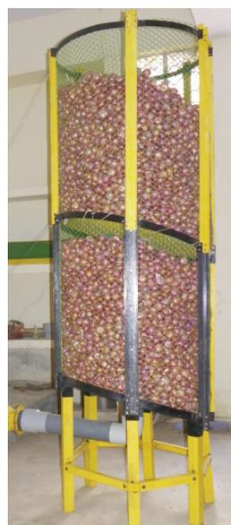
days in control storage. At the same time losses are 26.66% weight loss, 14.20% rotting and 5.88 % sprouting reported by other studies after 120 days storage. The structure is rust proof and hence expected to have long life and durability due to FRP material as major construction material. The time required for filling up and emptying the storage cage is about 0.83 man-h/t and 0.4 man-h/t, respectively as compared to 1 man-h/t and 3 man-h/t in case of conventional Chawl structures.
