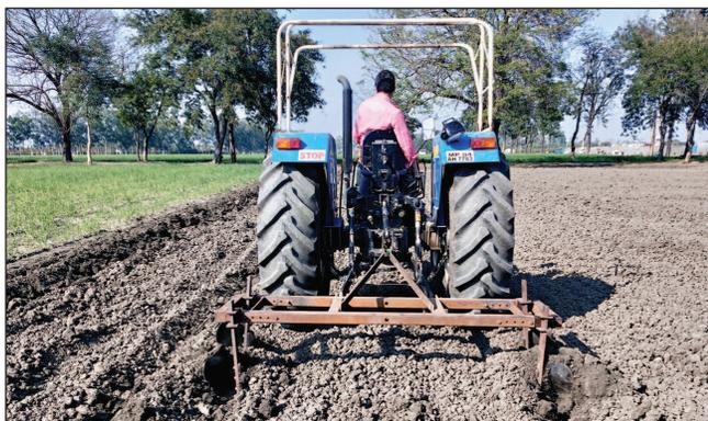
productivity and reduce drudgery by avoiding manual practice. The side trencher has adjustable width as well as depth. The width can be varied from 2.4-3.0 m as per the cropping pattern. The trencher can dig upto a depth of 300 mm.
