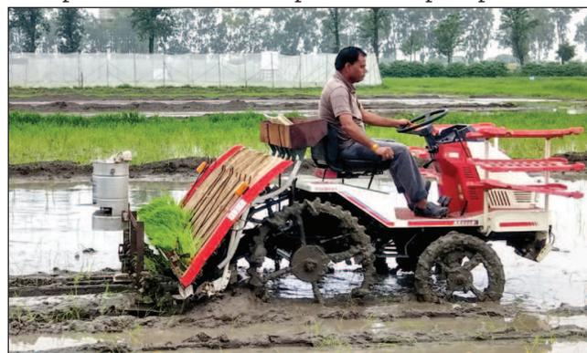
the time of transplanting. The performance parameters of rice transplanter with deep placement fertilizer applicator such as fertilizer application efficiency, field capacity and field efficiency are found to be 71%, 0.16 ha/h and 82%, respectively.
