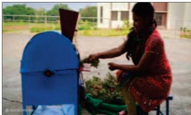
The threshing efficiency is about 95% with total pod losses with 5%. The cleaning efficiency is about 70%, which can be enhanced by adding a blower.
