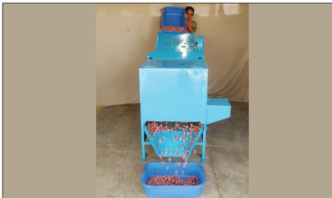
provided at the side for removal of the dust, dried and dead skin of onion. The maximum cleaning efficiency of 98% is obtained at 10.41m<sup>3</sup>/s air flow. The capacity of the cleaner is found to be 800 kg/h.
