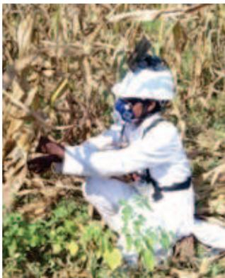
consists of 3 W solar panel, DC motor, fan and battery. A comparative study in similar climatic condition i.e. WBGT 28, 30 and 32 °C has been carried out with other popular head gear viz. bamboo hat, white pagdi etc. The result indicated that by using of headgear, the effect of heat stress significantly reduce thermal parameters (oral,
