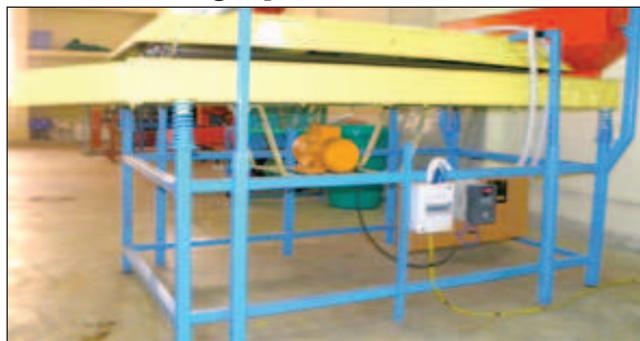
of IR heating module. The system is suitable to adjust spacing in the range from 25 mm to 120 mm. Developed prototype is suitable for infrared treatment of all types of free flowing grains at desired experimental conditions. Based on type of grains the machine has a output capacity of about 200-250 kg/h.
