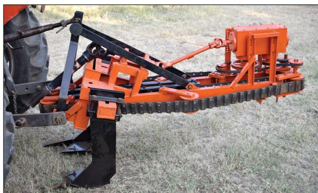
breaking blade through suitable belt drives. The cost of the equipment is Rs. 80,000. The effective field capacity of the planter is 0.22 ha/h. The cost of operation of the equipment is Rs. 2,265/ha and it saves 82% cost as compared to manual harvesting.
